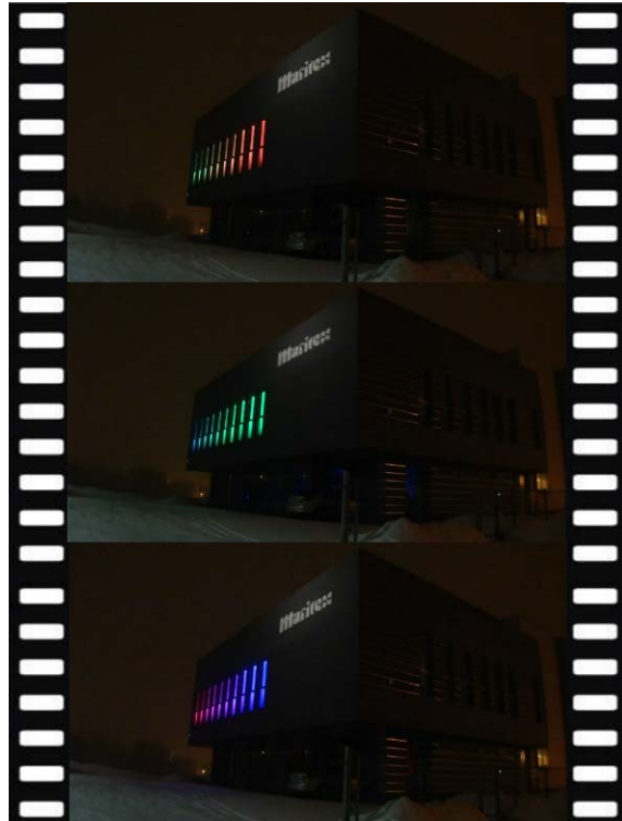
Fig. 5. RGB Lighting of NIVISS office using 30 channels DMX Controller [8]
