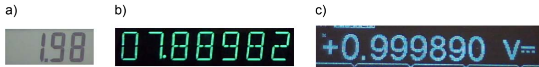
Fig. 1. Different kinds of the displays considered during development of the software: a) 7-segment display, b) 14-segment display, c) graphic display
