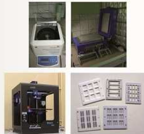
Spin-coater and doctor-blade (top) and 3D printer along with constructed mask for electrode evaporation (bottom)
