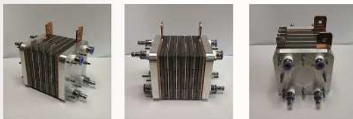
3x Fig. 1. The real picture of short, low-power PEMFC stack designed at Electrotechnical Institute
